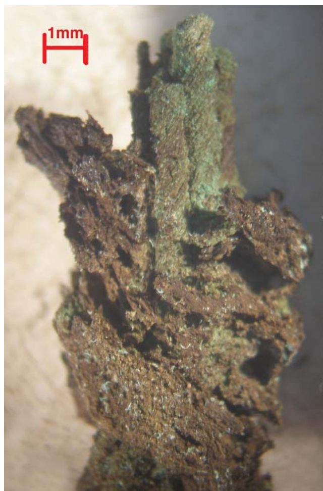
Fig. 10. Starting/side edge of textile Y3. The warps have the characteristic green colour of copper oxidation products, whereas the wefts have a brown colour. Scale bar 1 mm (© authors).
