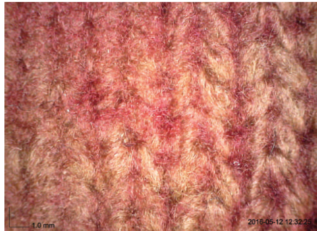
Fig. 3. The red pile on a knitted cap lining at the Museum of London (A6346) showing the yarn is paler than the pile and two unplied threads forming each stitch.
