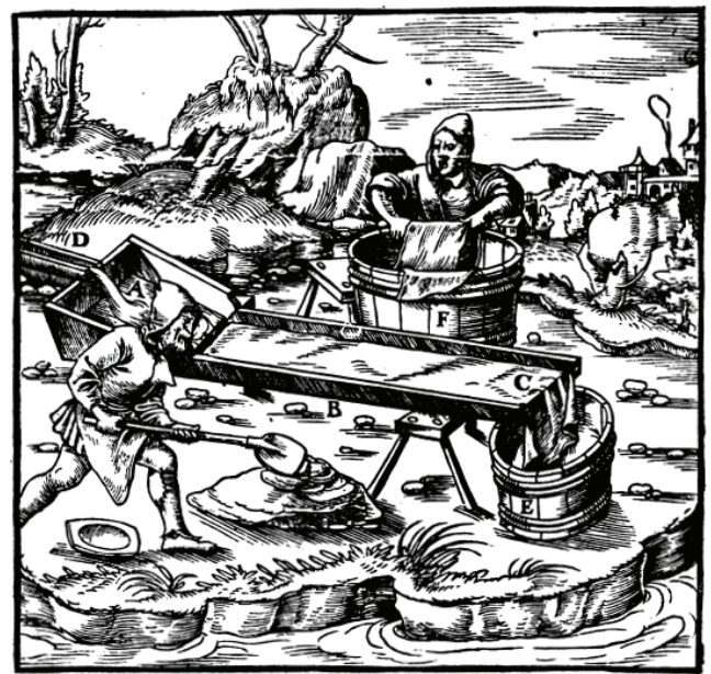
Fig. 17. Etching from De re metallica , illustrating the sluice. A: Top of the table, B: Table, C: Rag (textile), D: Pipes, E: Collection tank for rubbish, F: Tank for textile washing (After: Agricola 1530, 264).
