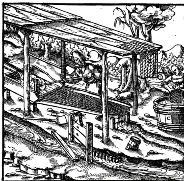
Fig. 19. Etching from De re metallica , illustrating the sluice. A: Taut net, B: Net, C: Tank for textile washing (After: Agricola 1530, 265).
