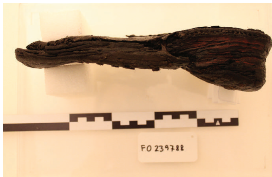
Fig. 4. XRF analysis showed that the colour on this heel contains lead. Lead is a component in the red pigment 'red lead' (Photo: Signe Groot Terkelsen).
