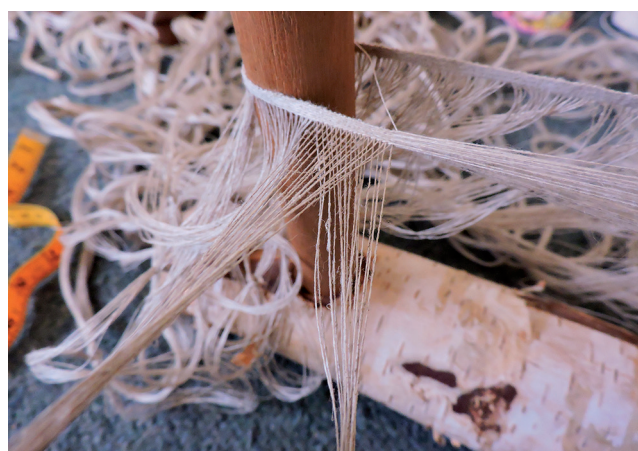
Fig. 7: Detail of the tablet-woven starting band showing the easy division of alternating threads (Image: Gwendoline Pepper)
