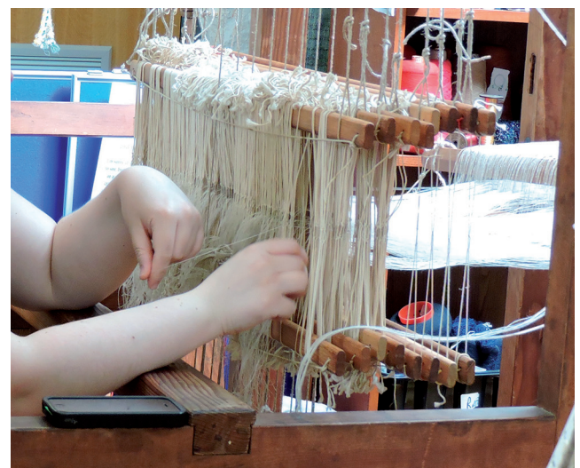
Fig. 16: Threading the heddles on the horizontal treadle loom (Image: Ruth Gilbert)
