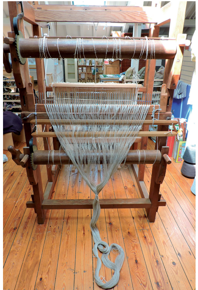
Fig. 14: The warp separated by lease sticks, attached to the warp beam, and spaced in the raddle ready for winding (Image: Gwendoline Pepper)
