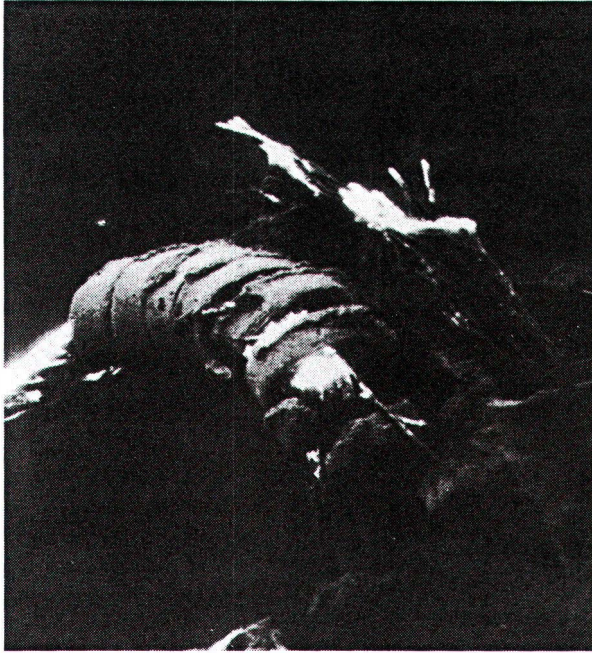
Figure 4 Flat silver strips (width 0.2 mm) spun around a silk core. (Ca.83x, scanning electron photomicrograph: Lena Holmquist Olausson).
