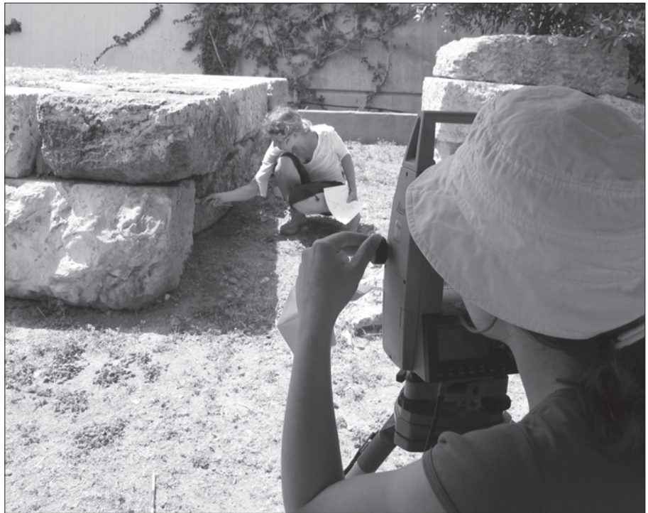
Fig. 65 Surveyor 'shooting' directly to a feature aided by a 'pointer' (M. McCallum ©ZHP 2005).
