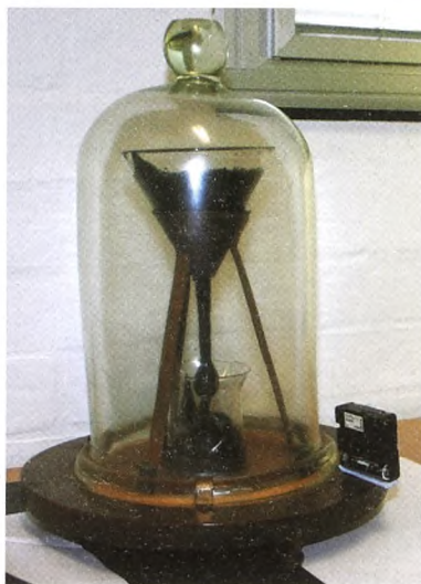
Figur 1. The Pitch Drop Experiment. Foto: Signe Riemer-Sørensen.
