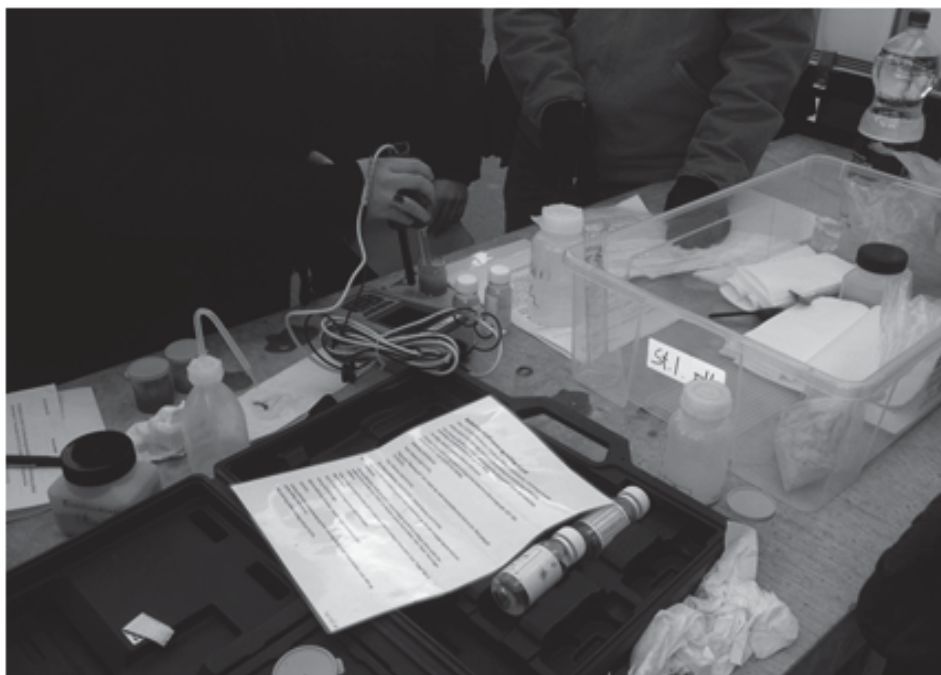
Fig. 12.3. Soil pH measurements and using field kits - which soil samples belong where ? Photo Pia Lund-Nielsen.
